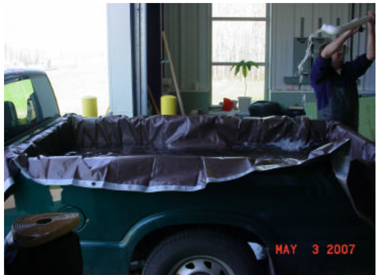
From Greg Fisher, NADF - Here are some photos of a quick fish hauler we rigged up to move some brook trout out of the hatchery over to the raceways. I though they made some interesting photos and a good idea that other hatchery/fish farms might be able use. We put a tarp in the bed of the truck filled with water and hauled fish a short distance. You need to be careful you don't go too fast or hit the brakes hard or the fish slosh out!!!!
